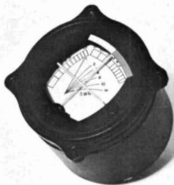
Photo of the I-101 converted to a direct-reading swr meter.
